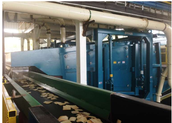
A modern BM&M Counterflow Chip Screen used in a wood chip screening application.
